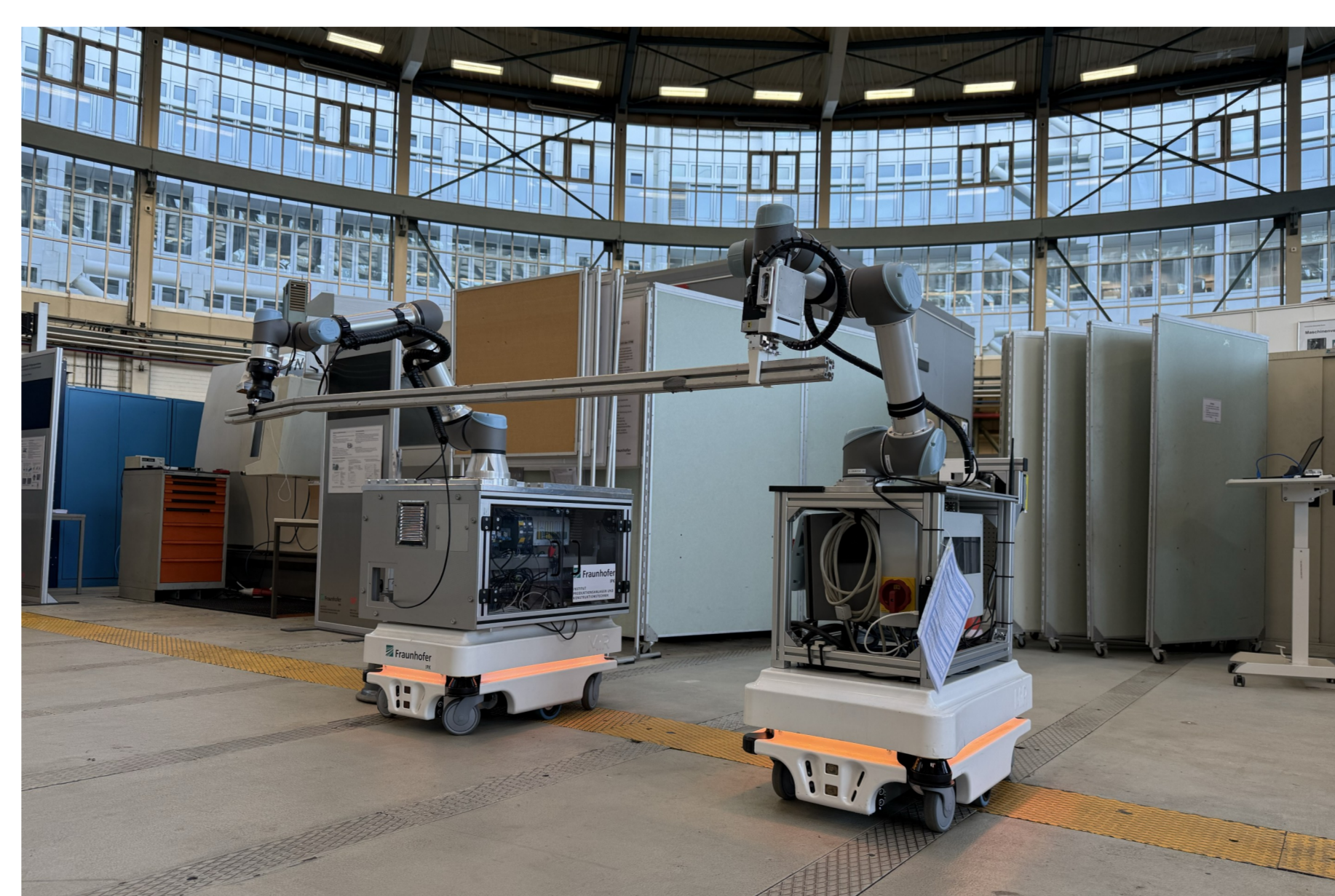
Beam lifting at the Fraunhofer IPK laboratory in Berlin.
